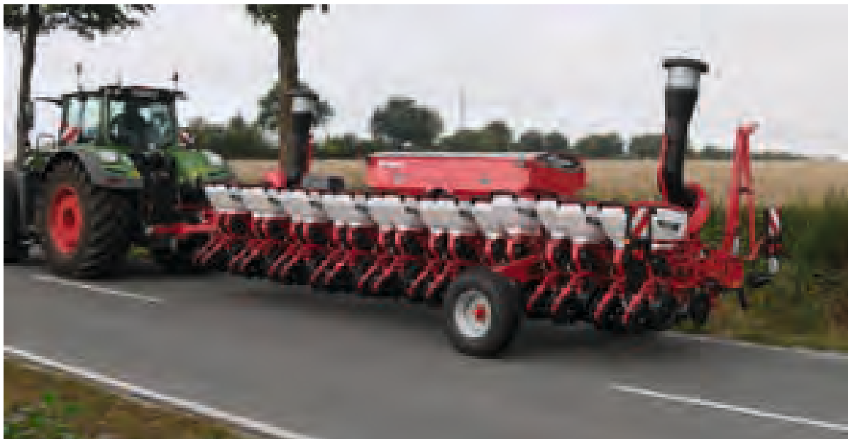
Optima RS Rahmen 18 reihig in Transportposition.
