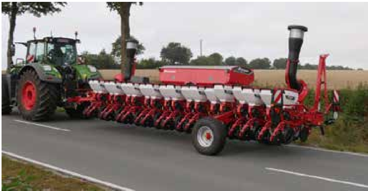
Optima RS Rahmen 18 reihig in Transportposition.
