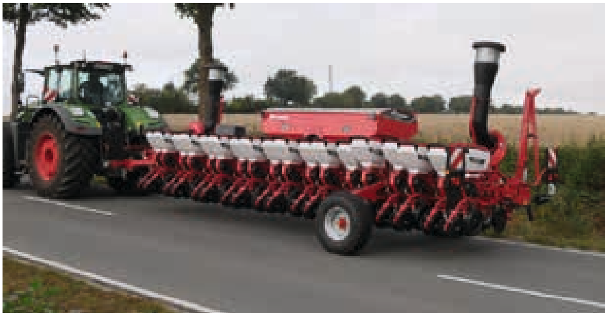
Optima RS Rahmen 18 reihig in Transportposition.
