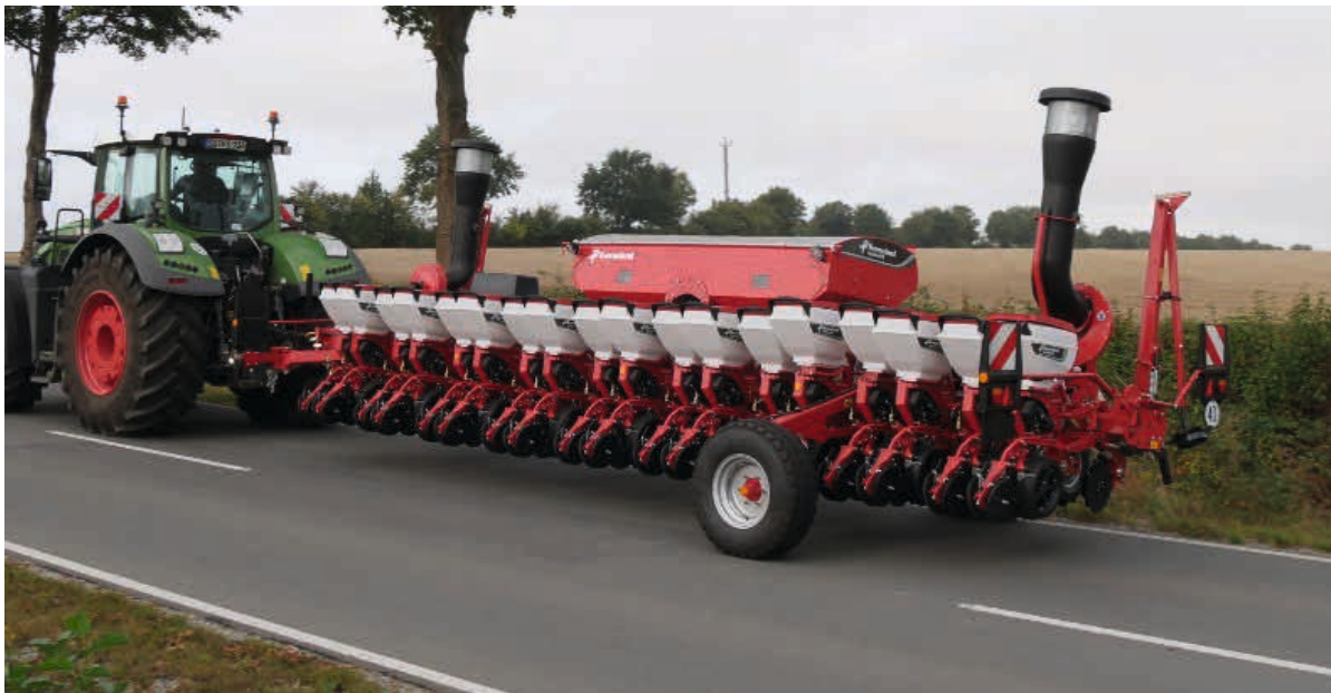
Optima RS Rahmen 18 reihig in Transportposition.
